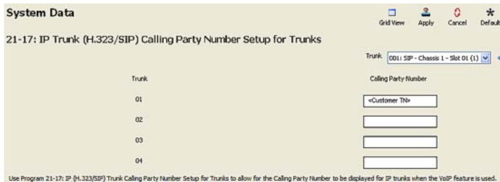
Figure 12 IP Trunk (H.323/SIP) Calling Party Number Setup for Trunks
